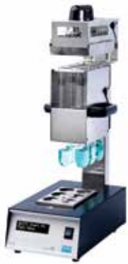
DK 6 6 position Performs batch digestion of up to 6 samples with 250mL test tubes - Ø 42mm ROWE CODE: ID0296
