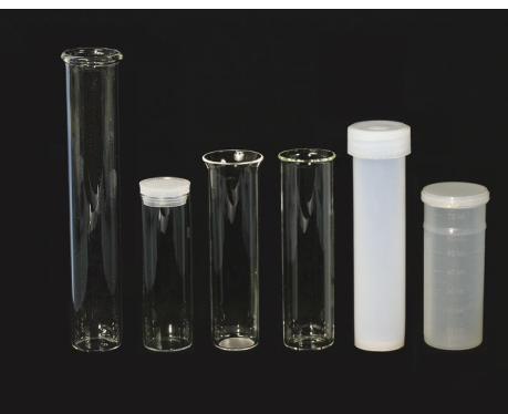
Example of typical special digestion vessels
