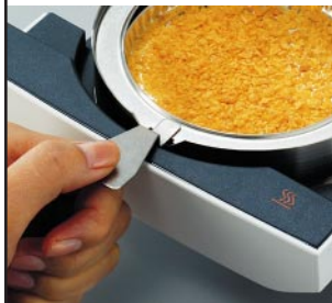
1 Insert sample holder. The sample drawer opens and closes at a keystroke.
