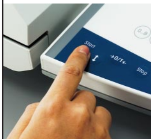
2 Press “Start”, the drawer closes automatically, the measurement begins.
